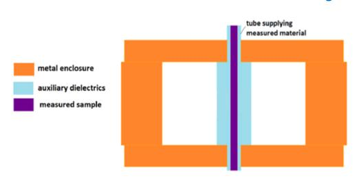
Schematic concept of the resonance cavity
