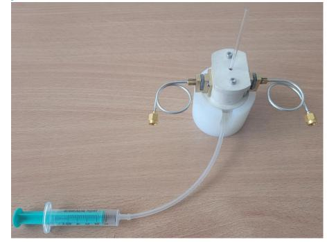
24-GHz Cavity resonator
